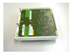
Figure 43: Bend Antennas carefully into vertical position
