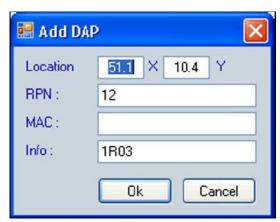
The RPN and Info values are automatically filled in. Ensure that the values are correct, and click **OK**. A DAP is created at the position you specified in the Add DAP dialog box.
