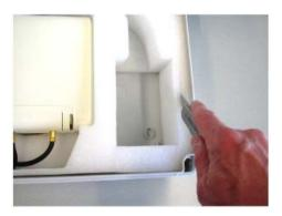
Figure 82: Cutting the foam to allow the antenna to fit into it, in the required position
