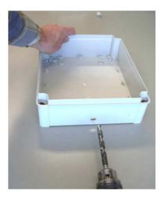
Figure 61: Drilling the hole (12 mm)
