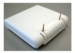
Figure 44: Antennas locked into Cover
