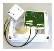
Figure 80: Connecting the cables to the 4720E
