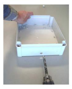
Figure 72: Drilling the hole (12 mm)
