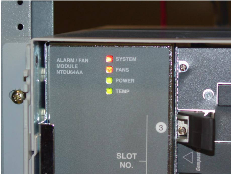
**Figure 3: Fan trouble LEDs**
