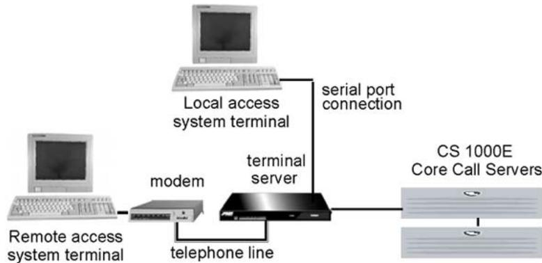
**Figure 1: Avaya CS 1000E local and remote access system terminals**
