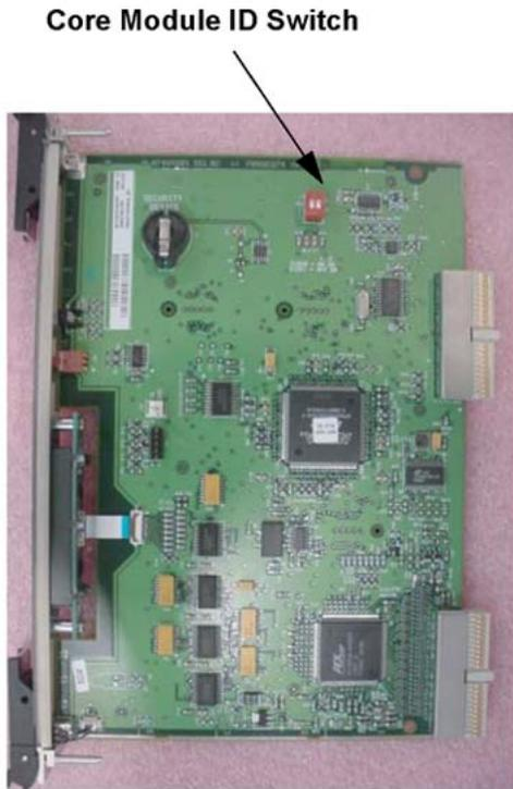
**Figure 7: Core Module ID switch**
