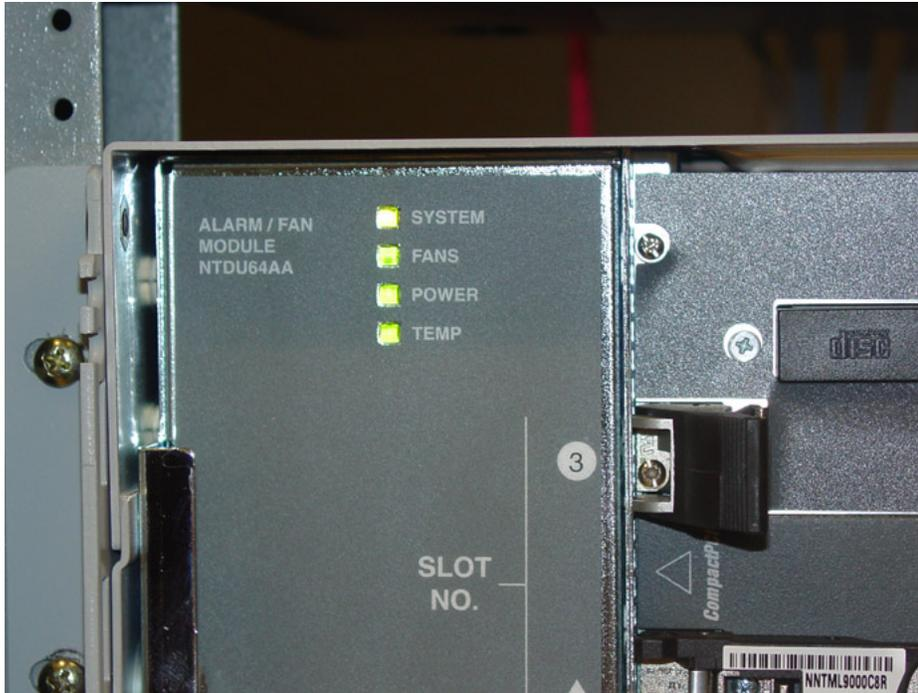
**Figure 2: Alarm/fan module status LEDs**
