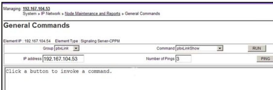
**Figure 53: Displaying pbxLink information in Element Manager**
