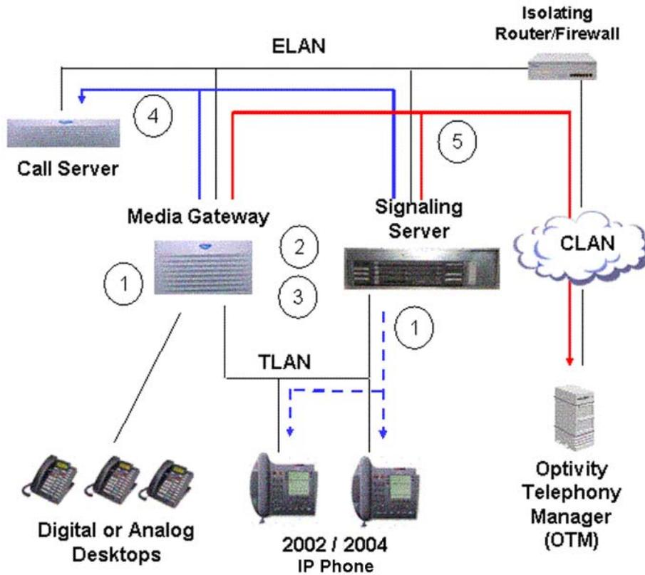
**Figure 52: Voice quality monitoring flow diagram**
