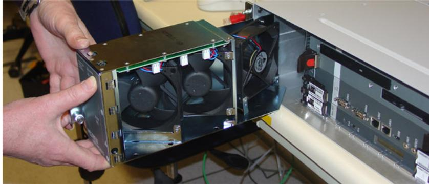
**Figure 44: Alarm/fan module**
