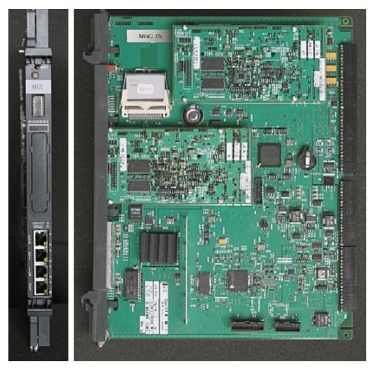
Figure 12: Media Gateway Controller card (NTDW60)
