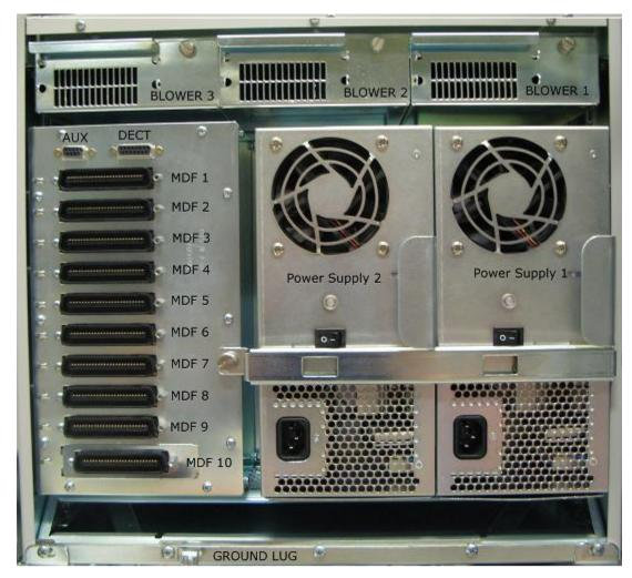
Figure 21: Rear components of the MG 1010
