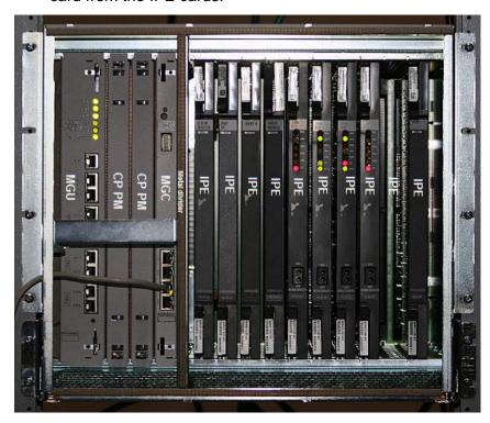
Figure 19: Front components in the MG 1010
