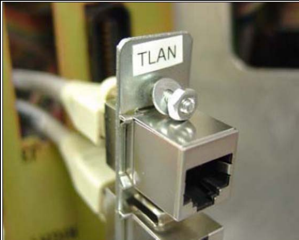
Figure 103 TLAN connection on Ethernet port coupler
