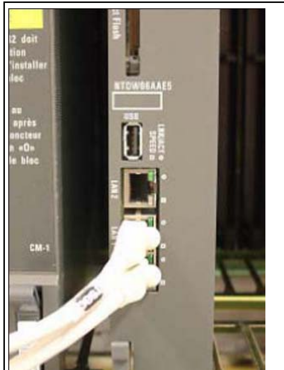
Figure 102 TLAN connection on CP PM faceplate
