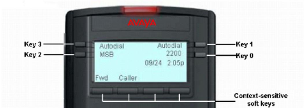
**Figure 325: Avaya 1220 IP Deskphone Programmable/DN Feature keys**
