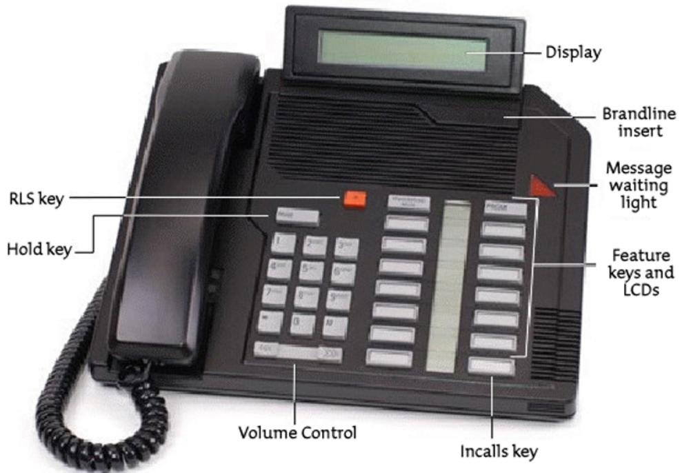
**Figure 365: Meridian M2616 Digital telephone layout**
