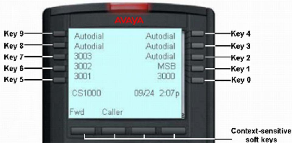
**Figure 328: Programmable/DN feature keys (first page)**
