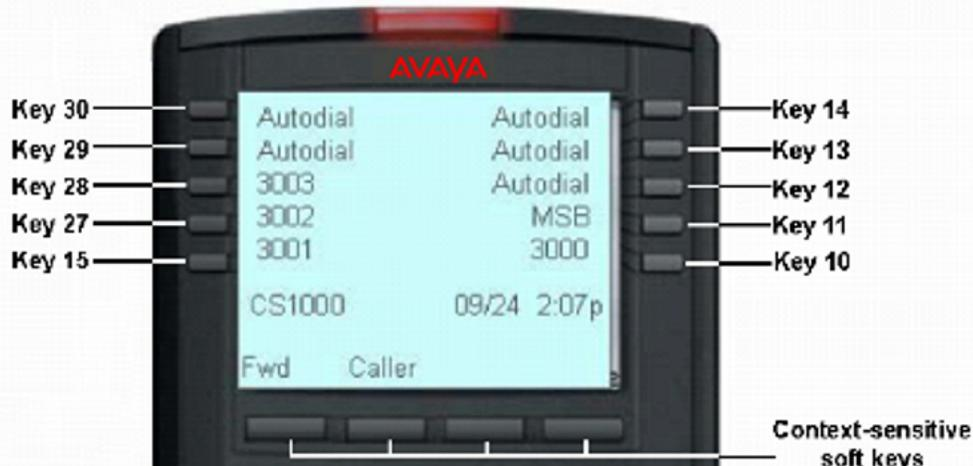
**Figure 329: Programmable/DN feature keys (second page)**
