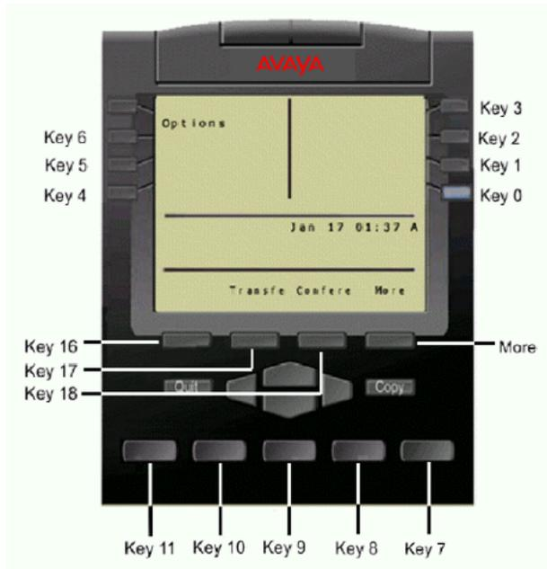
**Figure 388: Avaya 3905 Digital Deskphone with Feature Keys 0 - 11 and Soft Keys 16 - 18**
