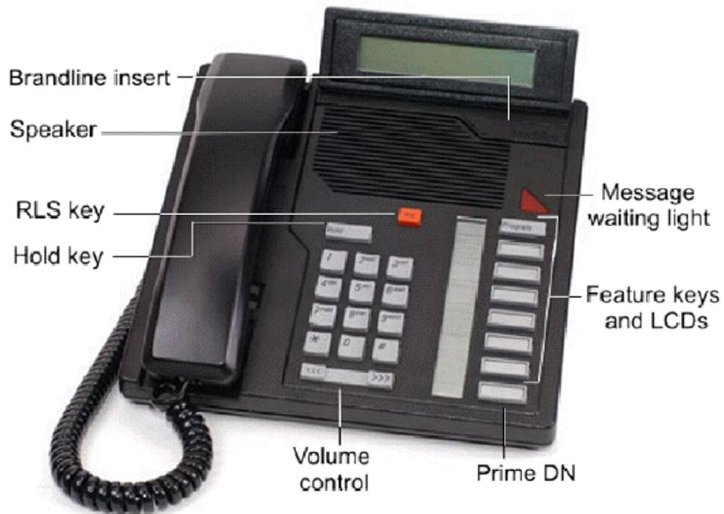
**Figure 363: Meridian M2008 Digital Telephone Layout**
