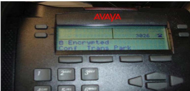
**Figure 1: Security icon and text indicator on an IP Phone 2002**
