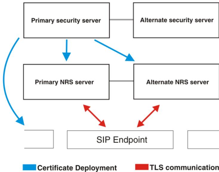
**Figure 14: SIP TLS with one security domain**
