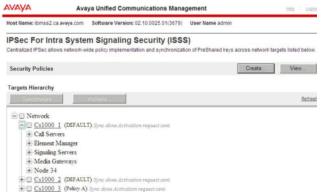
**Figure 2: IPsec for Intra System Signaling Security page in UCM**
