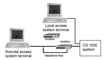
Figure 6: Direct modem and serial connections
