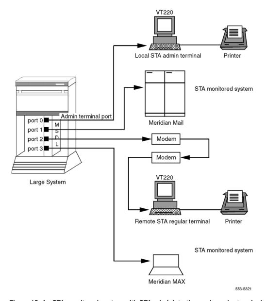
Figure 15: An STA-monitored system with STA administration and regular terminals
