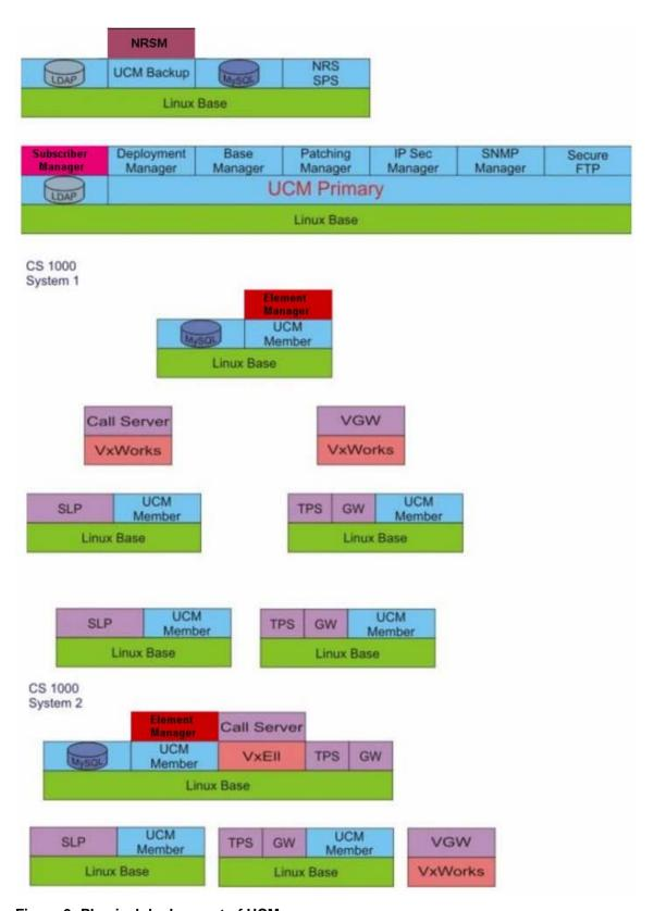
Figure 3: Physical deployment of UCM
