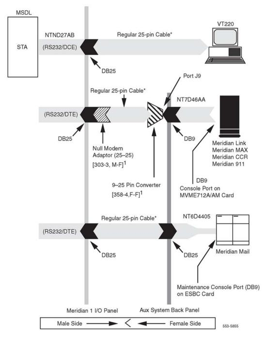
Figure 16: STA cable and connection information
