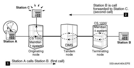
Figure 79: Anti-tromboning for Call Modification - DMS/System
