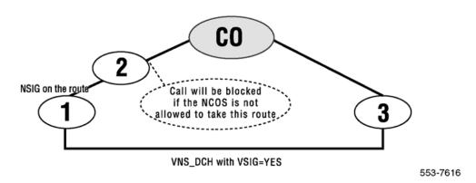
Figure 36: A scenario where the call is blocked, as NCOS is insufficient (VSIG = YES and SIGO is not set to STD)
