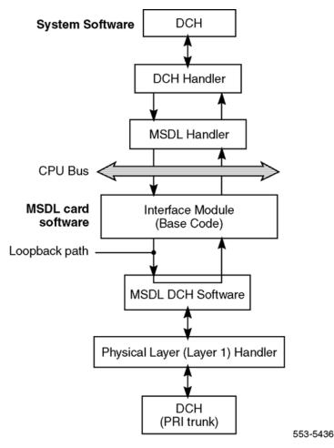
Figure 132: Local loopback test (NT6D80)
