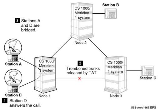
Figure 71: Tromboned trunks released by TAT
