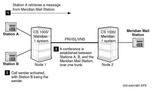
Figure 102: Call Sender operation with Network Message Services active
