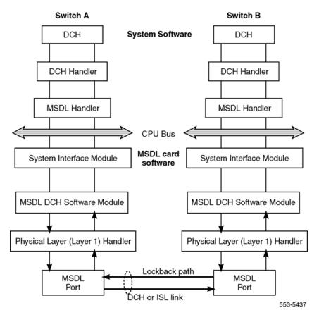
Figure 133: Remote loopback tests (NT6D80)
