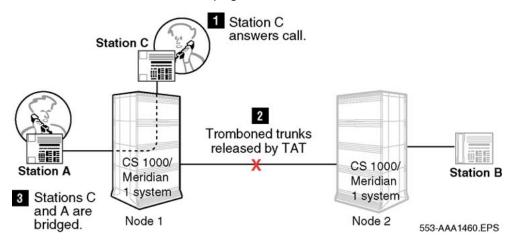
Figure 64: After TAT applied to tromboned trunks due to a call transfer
