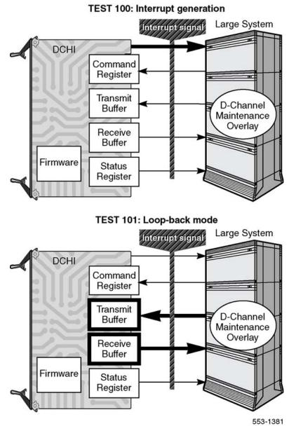
Figure 130: DCH tests 100 and 101
