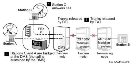
Figure 76: Results of anti-tromboning for NCRD (case 1), PBX/DMS
