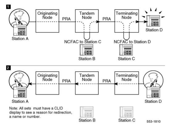
Figure 26: Tandem NCFAC intranode
