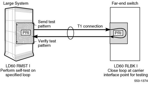
Figure 129: PRI remote loop-back and link diagnostic tests
