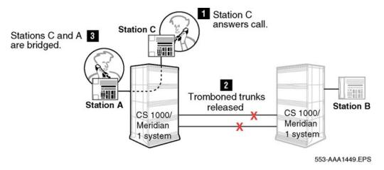
Figure 60: After Trunk Anti-Tromboning operation
