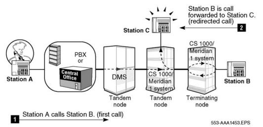
Figure 77: Anti-tromboning for NCRD (case 2), system/DMS
