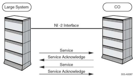
Figure 37: NI-2 B-channel Service messaging
