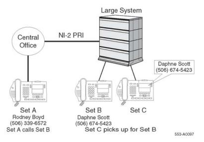
Figure 43: Call Pickup in a stand-alone environment
