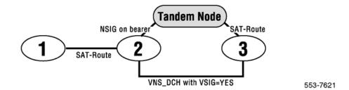
Figure 32: A scenario involving two SAT-Routes where VSIG = YES and SIGO is not set to STD
