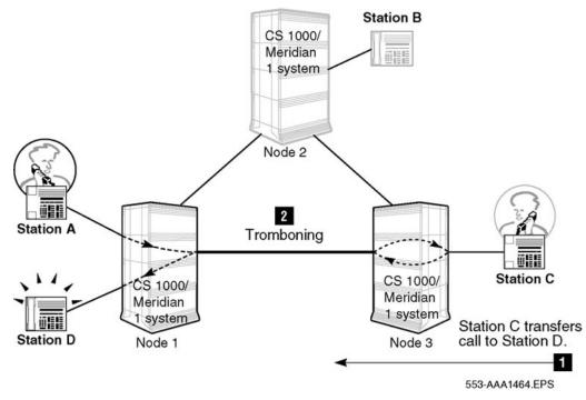
Figure 70: Tromboning of trunks after TRO-BA is applied
