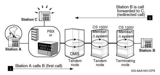
Figure 75: Anti-Tromboning for NCRD (case 1), PBX/DMS
