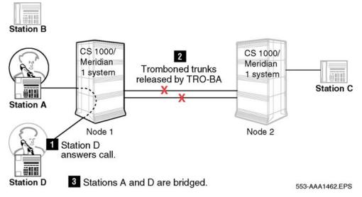
Figure 67: Tromboned trunks released by TAT
