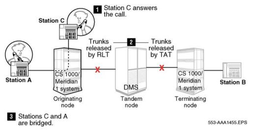
Figure 80: Results of anti-tromboning for Network Call Transfer - DMS/System
