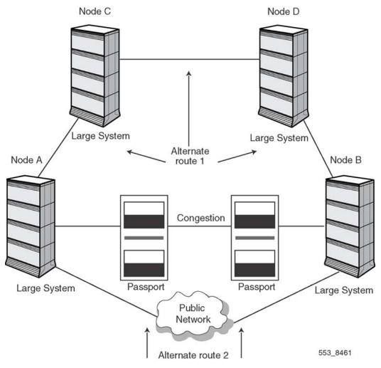
Figure 3: Example of System with Passport network
