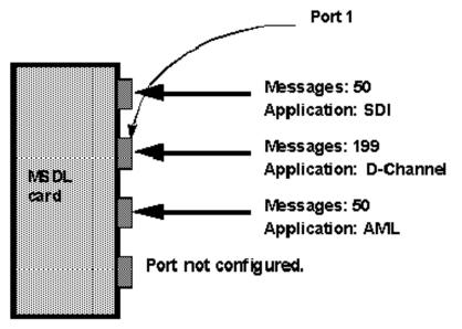
Total Messages per two seconds = 50 + 199 + 50 = 299 messages. If the 300th message arrives through port 1, it triggers a port overload check. On detection of a port overload, the port is locked; the incoming message count of the card is reduced by 200, bringing the card message count to 100 (50 SDI+ 50 AML).
