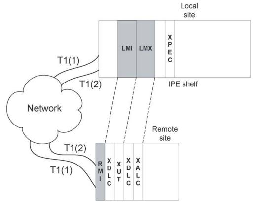
Figure 1: Mini-Carrier Remote (sample configuration)
