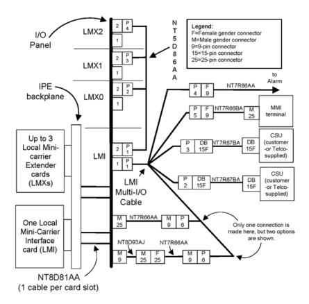
Figure 8: Cabling for a single Local Mini-carrier Interface card (LMI)
