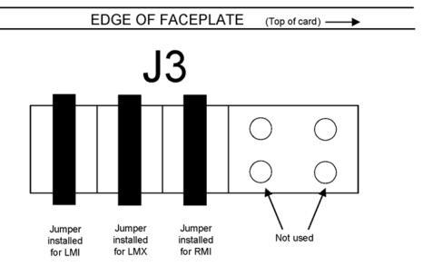
Figure 11: Jumper settings on MCR circuit packs.
