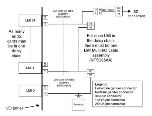
Figure 9: Cabling Local Mini-carrier Interface cards (LMIs) in a daisy chain
