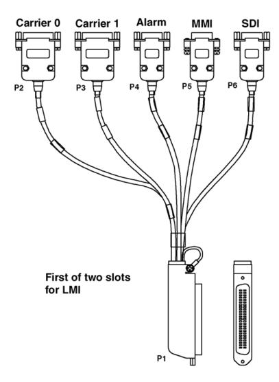
Figure 5: LMI Multi-I/O cable assembly (NT5D85)
