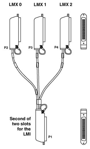
Figure 6: LMI/LMX Multi-I/O cable assembly (NT5D86)
