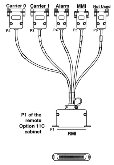
Figure 7: RMI Multi-I/O Cable Assembly (NT5D87)
