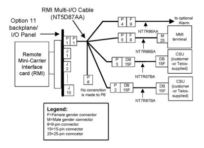
Figure 10: Remote Mini-carrier Interface cabling
