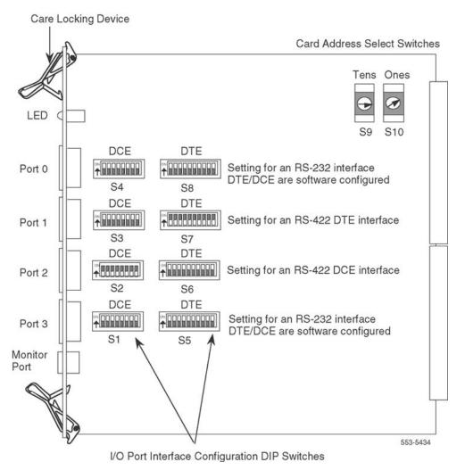
Figure 93: MSDL switch setting example
