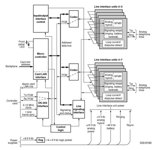
Figure 23: OPS analog line card - block diagram
