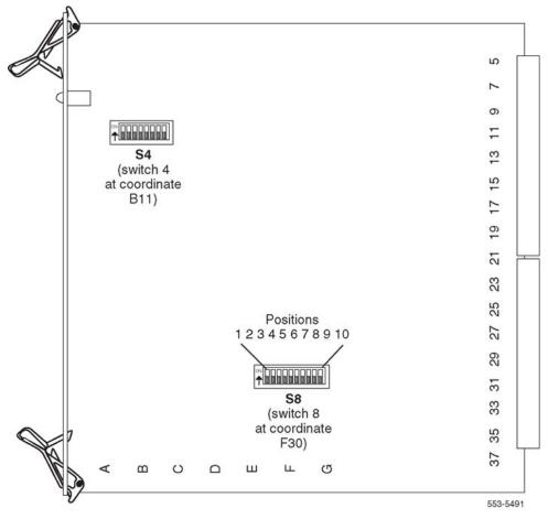
Figure 19: Circuit card grid
