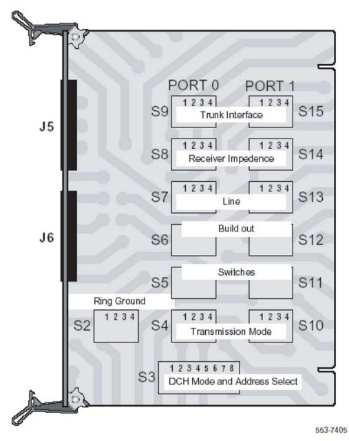
Figure 83: Dip switches for NT5D97AA/AB
