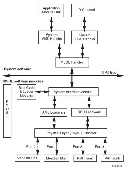
Figure 92: MSDL functional block diagram
