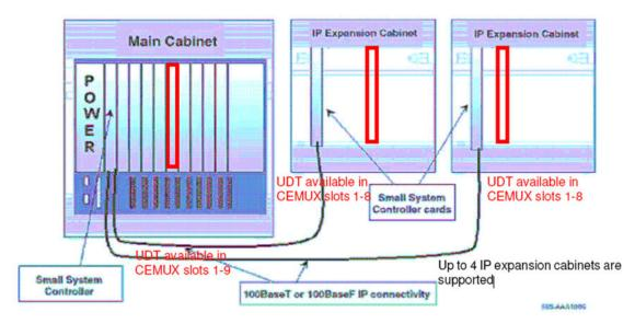
Figure 154: UDT card positioning in Avaya CS 1000M Cabinet/ Meridian 1 PBX 11C Cabinet
