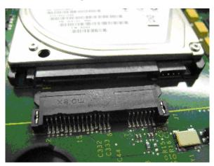
Figure 169: CP MG card hard drive connector
