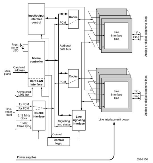
Figure 2: Typical IPE analog line card architecture
