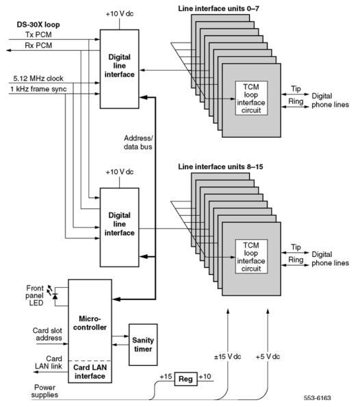
Figure 101: Digital line card - block diagram
