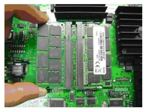
Figure 184: Inserting a memory module in CP PM card
