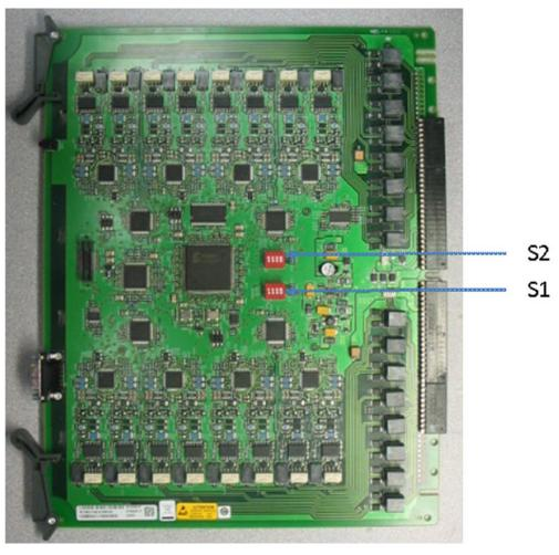
Figure 99: Analog message waiting line card - switch locations
