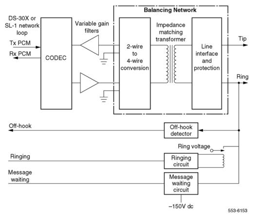
Figure 4: Typical analog line interface unit block diagram
