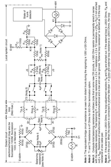
Figure 142: 4-wire DX signaling
