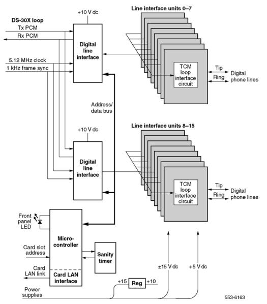
Figure 103: Digital line card - block diagram
