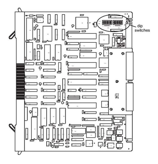
Figure 48: LEI card - E1 protocol dip switch locations
