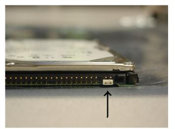
Figure 177: CP PM hard drive jumper
