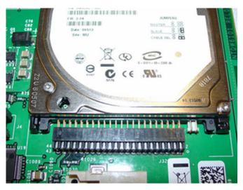
Figure 178: CP PM hard drive and connector J32
