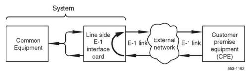
Figure 40: MMI network loopback test
