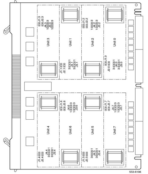
Figure 135: Universal trunk card - jumper locations for NT8D14BA and NT8D14BB Release 9 and below
