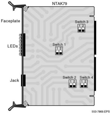
Figure 153: NTAK79 card with switch locations
