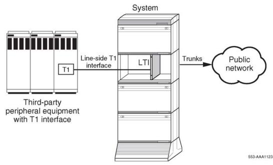
Figure 41: Lineside T1 interface connection to IPE
