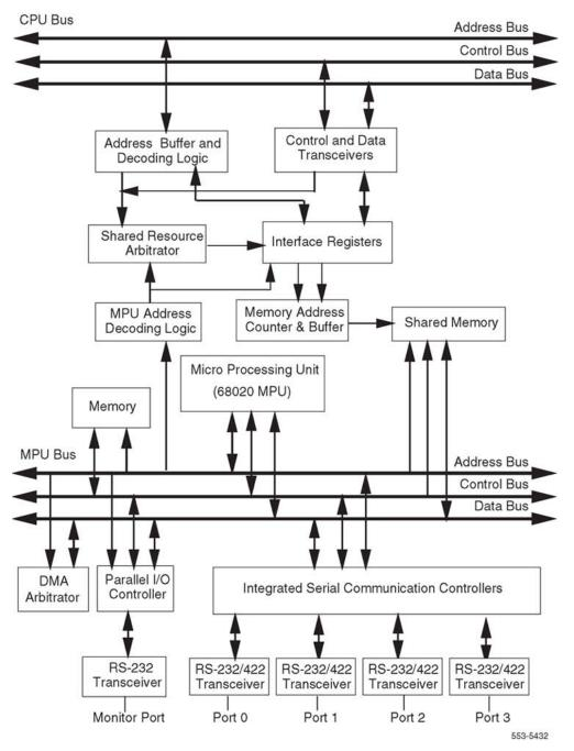
Figure 91: MSDL block diagram
