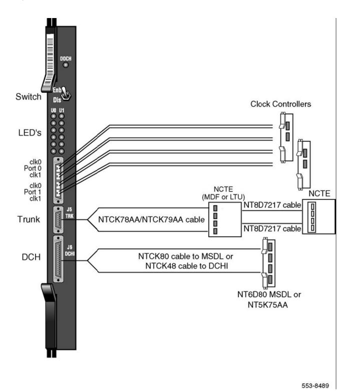
Figure 81: DDP2 cable for systems with an I/O panel
