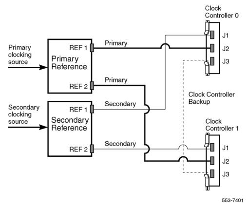
Figure 85: Clock Controller primary and secondary tracking
