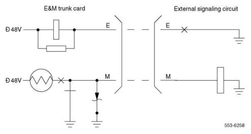
Figure 140: E and M Type I signaling
