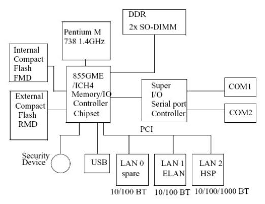
Figure 175: CP PM high level hardware block diagram
