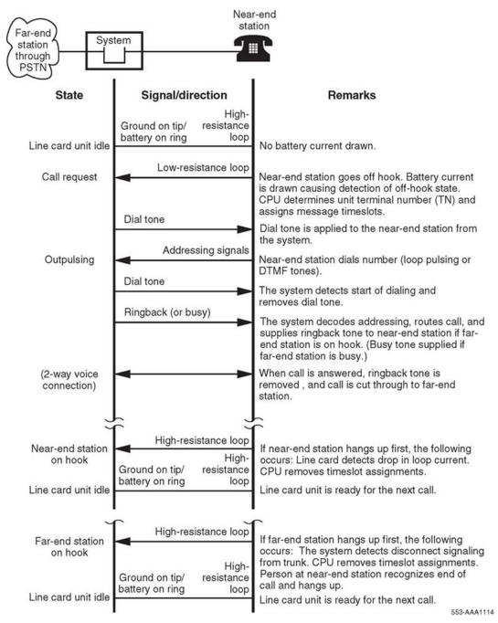
Figure 7: Call connection sequence - near-end originating call
