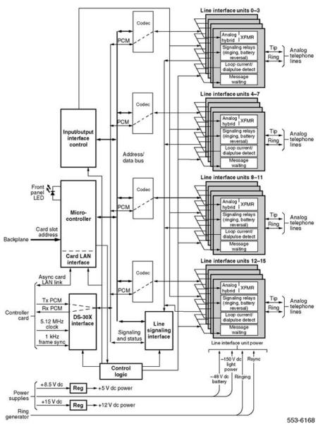
Figure 106: Analog message waiting line card - block diagram
