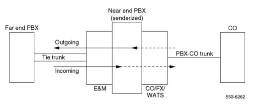
Figure 144: Signaling orientation for tandem connection between E and M and CO trunks
