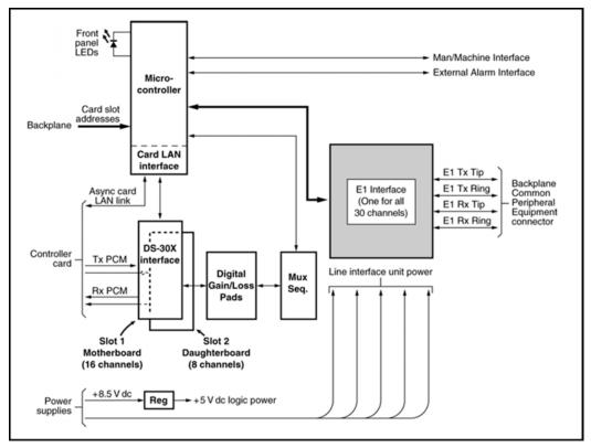
Figure 46: LEI card - block diagram
