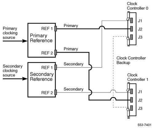
Figure 86: Clock Controller - Option 1
