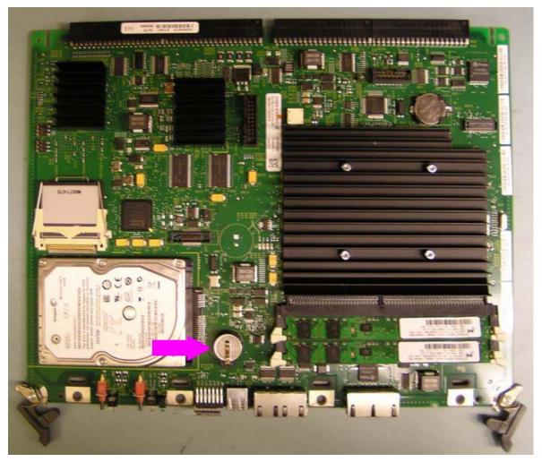
Figure 170: CP MG Security Device (Dongle)
