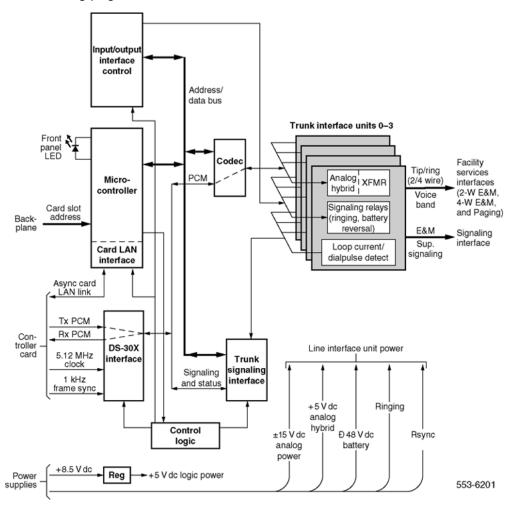
Figure 139: E and M Trunk card - block diagram
