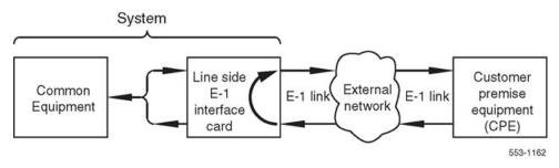
Figure 69: MMI Network loopback test
