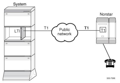
Figure 43: Lineside T1 interface connection to Norstar system
