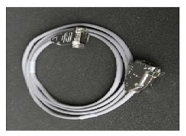
Figure 34: MGC DECT Clock Reference Cable Connecting MGC DECT Clock Reference Cable
