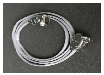
Figure 50: MGC DECT Clock Reference Cable
