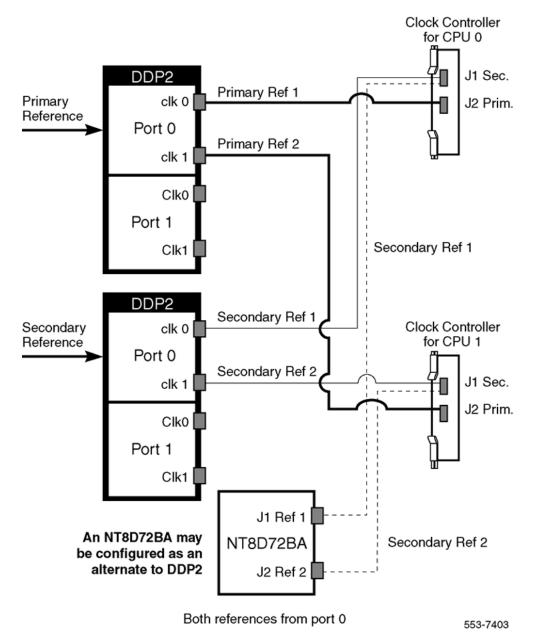
Figure 87: Clock Controller - Option 2
