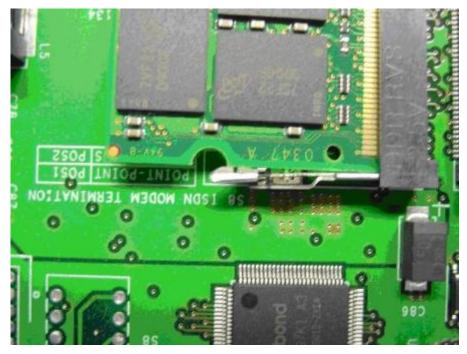
Figure 186: Incorrectly aligned memory module
