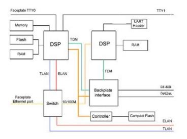
Figure 193: Voice Gateway Media card block diagram
