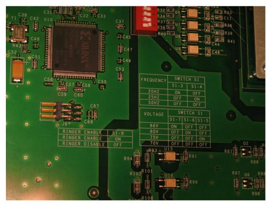
Figure 199: MGU dip switch settings
