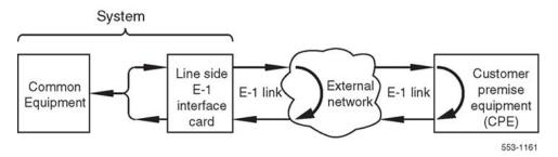
Figure 68: MMI External loopback test
