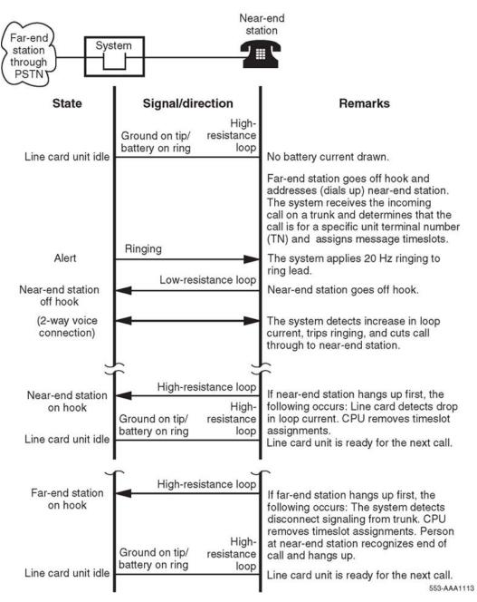
Figure 6: Call connection sequence - near-end station receiving call
