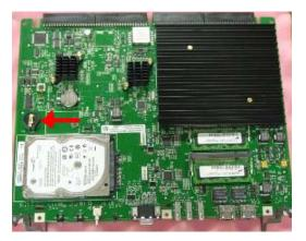
Figure 174: CP DC security dongle
