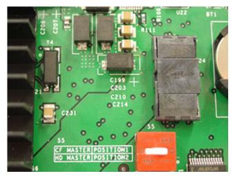
Figure 180: CP PM Signaling Server FMD dip switch
