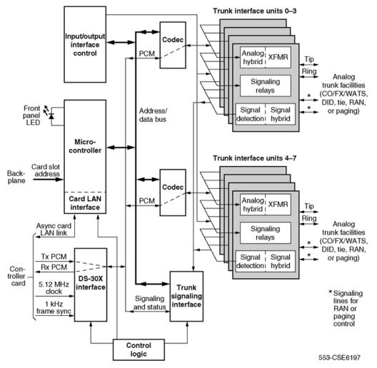
Figure 110: NT8D14 Universal trunk card - block diagram
