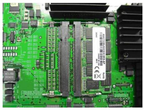
Figure 183: CP PM card with empty memory slot
