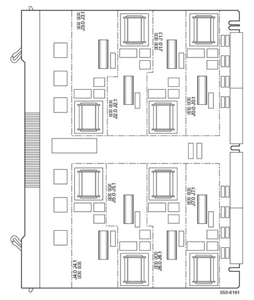
Figure 25: OPS analog line card - jumper block locations
