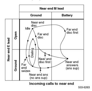
Figure 145: E and M Type I signaling patterns - originating party release
