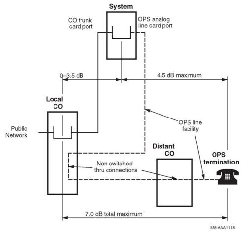
Figure 26: Traditional OPS application configuration
