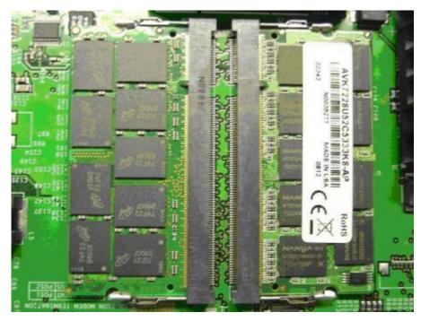
Figure 187: Correctly aligned memory module
