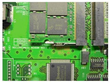
Figure 185: Fastening memory module in CP PM card
