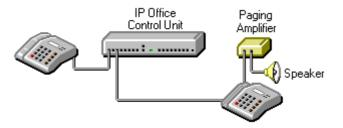
The external loudspeaker system must be CE marked to indicate compliance with the EMC (EN41003) and Low Voltage (EN60950) directives.
