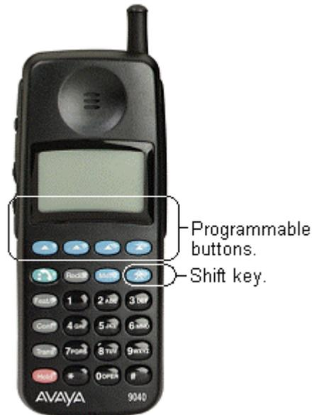
9040 display buttons labeled **1** to **4** correspond with IP Office user buttons 1 to 4. 9040 display buttons labeled **A** to **D** correspond with IP Office user buttons 8 to 11.
